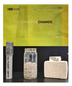
Example of one of the winners of the latest challenge on plastics: PVC waste from construction transformed into new insulation materials (MgO Systems)
