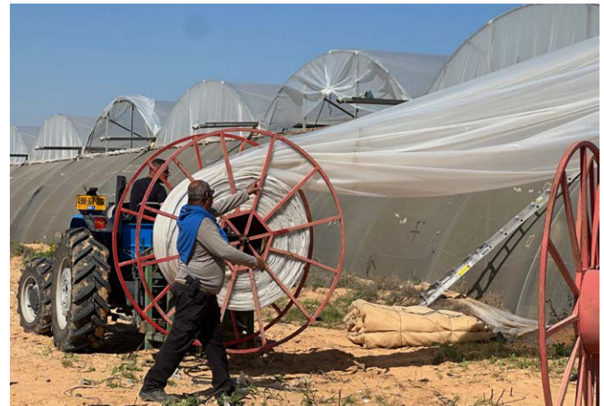
Image: Plastic cover films rolling equipment: Tractor, Winder, and Drum
